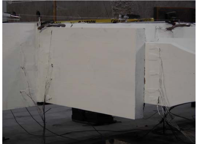
Figure 11. As predicted by our nonlinear finite element analysis (Naeim, 1999), at low amplitude cycles there would be some rise in stress along the tip of the cover plate that would subside as the specimen would go into nonlinear range. That is exactly what happened. This picture is taken at yield displacement.
