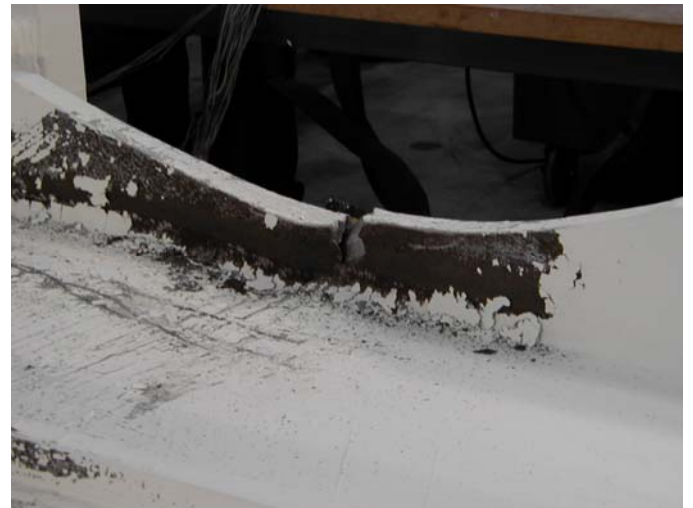
Figure 16. Finally, at 5\delta_y (5.4% plastic rotation, 6.8% total rotation) failure of 36-1 specimen starts by tension failure of the bottom flange at the center of RBS and propagates into the web. Specimens 40-1 and 40-2 stayed course as the actuators ran out of stroke at plastic rotations exceeding 7%.
