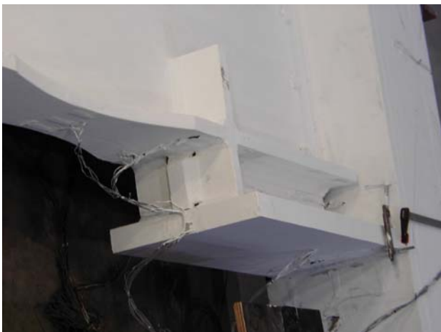
Figure 9. Whitewashed and instrumented bottom RBS and haunch.
