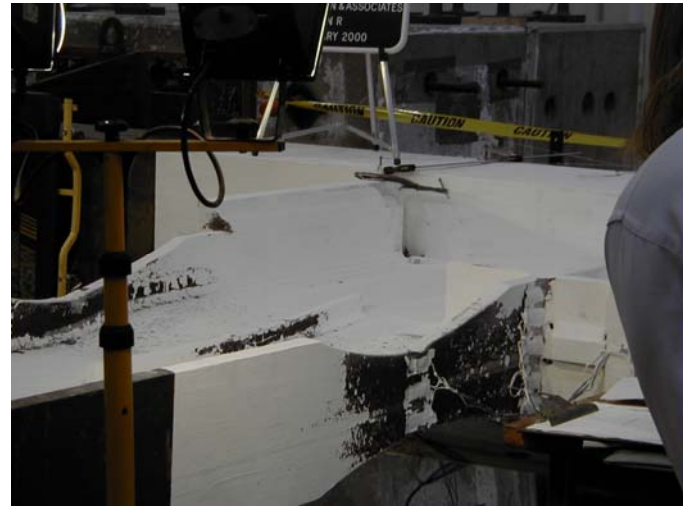
Figure 15. At the end of regulatory testing or 4% plastic (6.8% total) the specimen (36-1 showed here) is still showing increasing capacity and no loss of stiffness is present. Plastification of RBS flanges, buckling of the beam web and some local buckling of the RBS flange may be observed.
