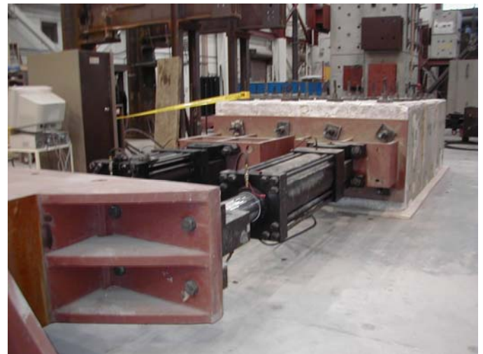
Figure 6. The two actuators used in series to force cyclic displacement at the end of the beam.
