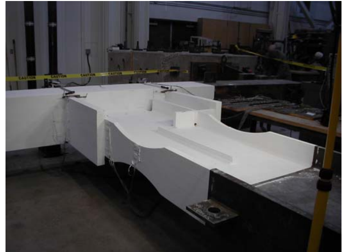
Figure 5. The 36-1 specimen in place ready for testing. The areas of concern are whitewashed to show possible signs of distress.
