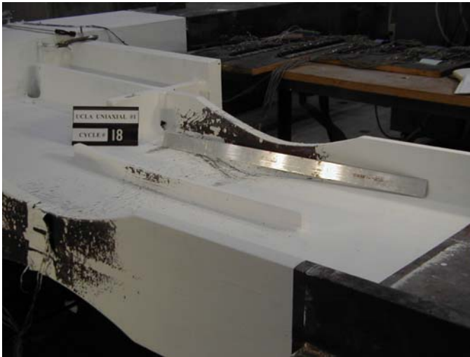
Figure 13. At the end of 3\delta_y cycles or 2.7% plastic rotation web buckling may be observed, but no strength reduction is yet noticed (photo of specimen 36-1).
